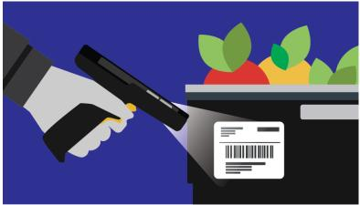
Items, materials, or ingredients used at each production stage, including temperature data, are recorded using fixed industrial or handheld scanners, creating batch numbers for tracing, compliance and recall purposes.
