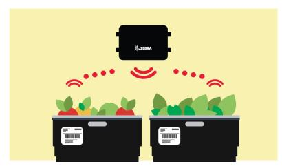
As components or raw materials arrive, RFID readers automatically register them into your ERP system. Electronic sensors validate that temperature thresholds have not been exceeded, and your team can also scan items at receipt, recording item stock and location.
