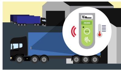
Electronic sensors and data loggers can be added to shipments, for example fixed to pallets or inside trailers. As well as helping to monitor quality, temperature data can be shared at the point products are handed off across the supply chain, to validate that excursions have not occurred.
